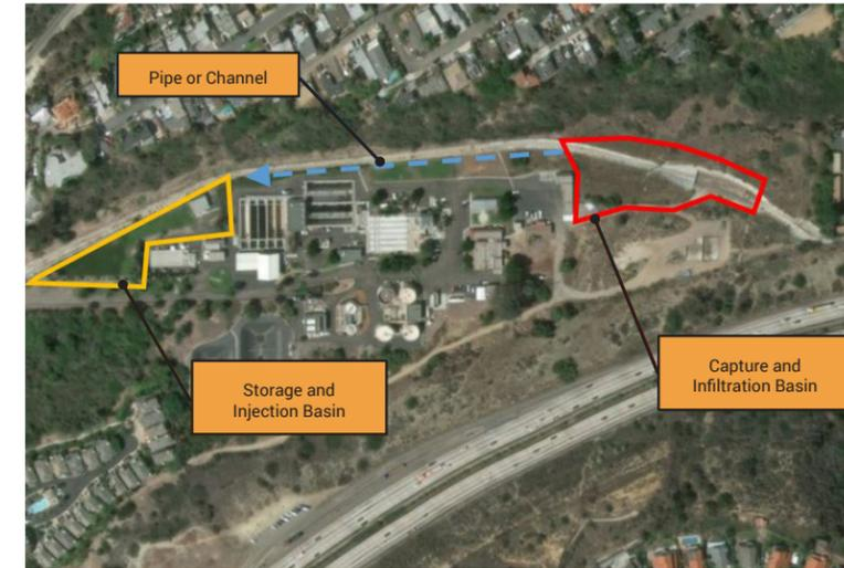
SEWRF Stormwater Capture Elements
