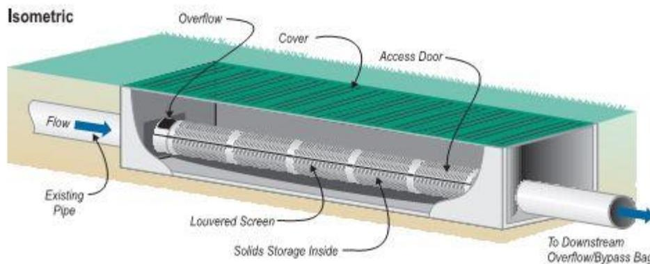
FIGURE 5 FULL CAPTURE DEVICE - CONCEPT LINEAR RADIAL CONFIGURATION 1 (CALTRANS OCTOBER 2003)
