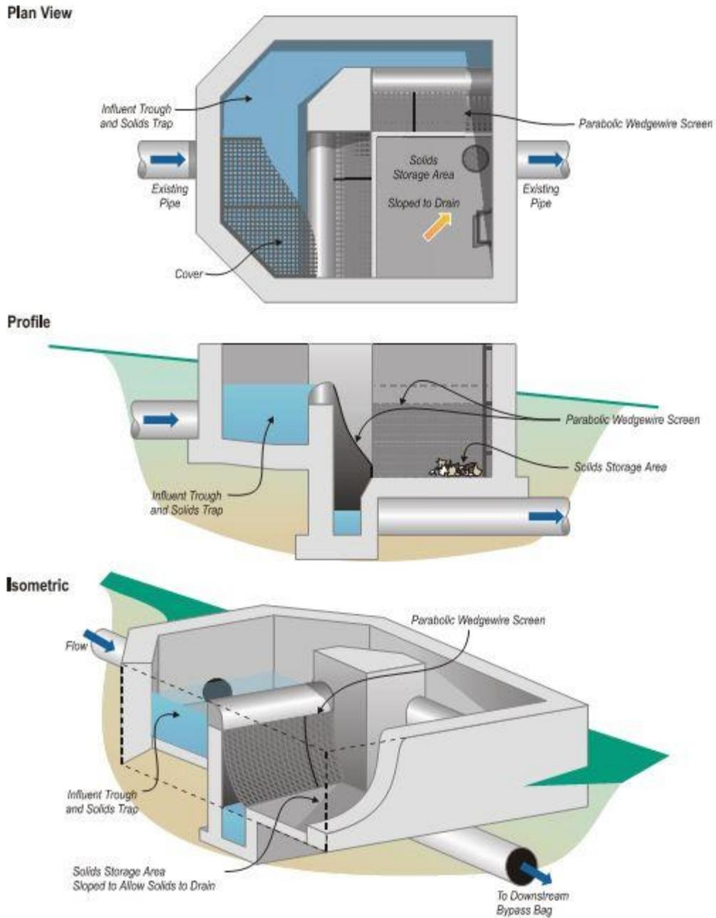
FIGURE 6 FULL CAPTURE DEVICE - CONCEPT INCLINED SCREEN CONFIGURATION 1 (CALTRANS OCTOBER 2003)
