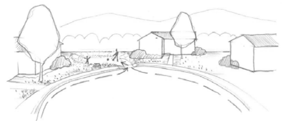
Bioretention facility configured and planted as a lawn/ play area.
