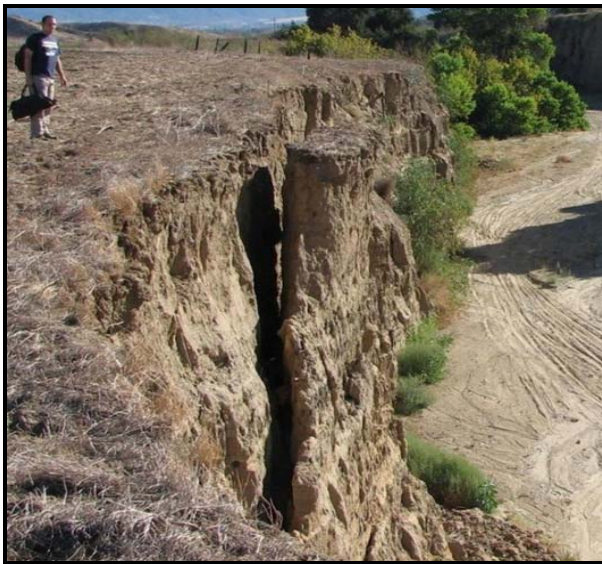
Figure 8. Planar/Slab failure with tension cracks, exhibiting cohesive consolidated banks, at San Timetao, San Bernardino County, CA (a) and Acton, Los Angeles County, CA (b).
