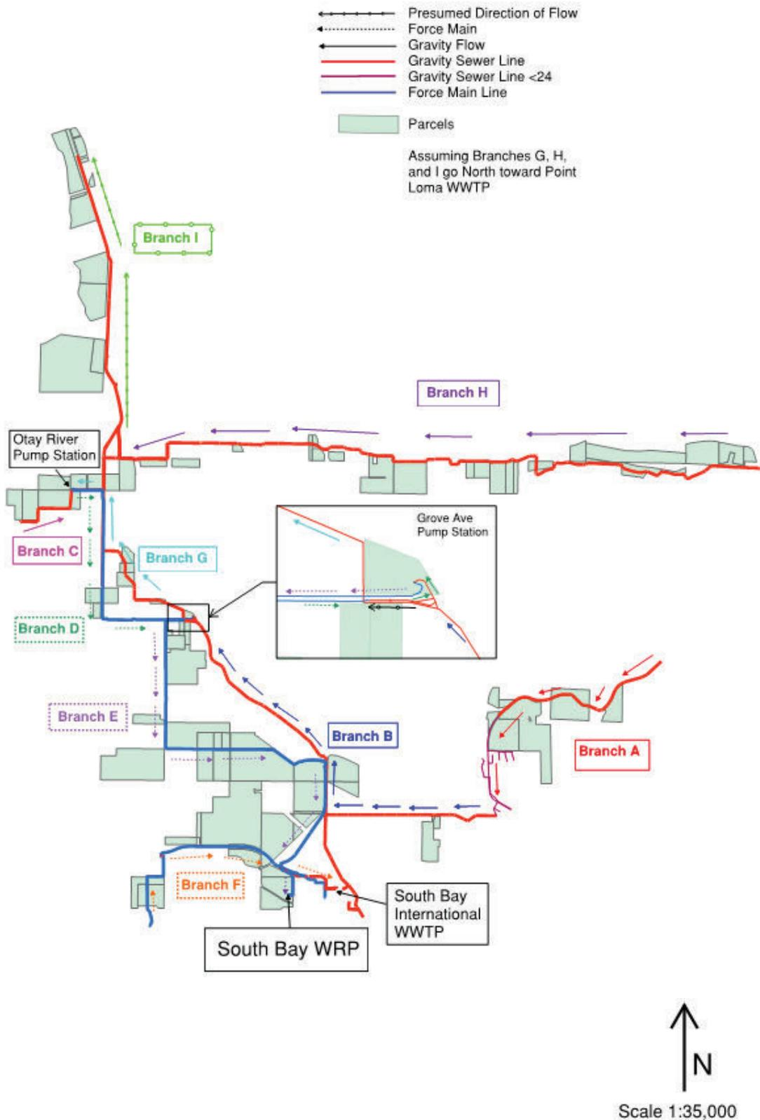
**FIGURE 1 – SBWRP Sewershed, showing major sewer lines, force mains, and stormwater parcels used for volume and capacity evaluations.**
